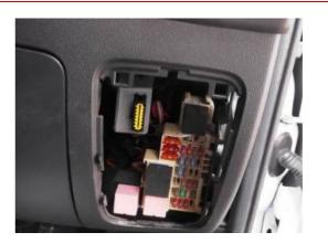
2. Locate suitable constant and ignition feeds and route wiring to slot above radio. Suitable power and ground connections may also be obtained from the power plug at the rear of the radio. Connect A1 +VE to Tachograph through 1 Amp fuse.
