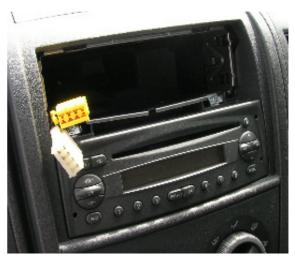
4. Route all cables to slot above radio and ensure the tachograph can be removed from its housing with all of the connectors attached.
