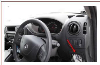
1. Remove O/S lower panel to gain access to the fuse board. Locate VU in slot above the radio.
