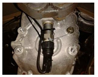
3. Remove blanking plug and install Kitas 2+ Sensor 9954-250 included in supplied kit. Route cable through a suitable bulkhead grommet to the tachograph location point.
