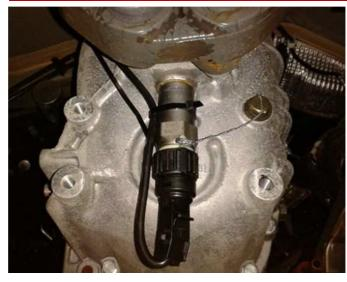
REMOVE REAR GEARBOX BLANKING PLUG AND IN-STALL 9954-250 KITAS 2+ SENSOR SUPPLIED.
