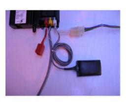
2. The cable harness is connected directly in line with the tachograph power cable when connecting to the tachograph as shown.
