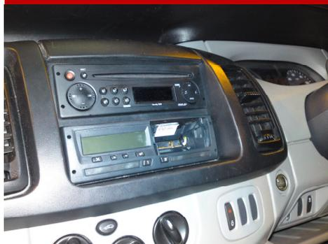
INSTALL THE TACHOGRAPH IN THE COIN TRAY BELOW THE RADIO AS SHOWN LEFT.
