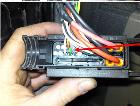
SUITABLE POWER AND GROUND CONNECTIONS CAN BE LOCATED AT THE FUSEBOX OR AT THE REAR OF THE RADIO, ENSURE THE POSITIVE FEED TO A1 ON SE5000 IS TERMINATED VIA 1 AMP FUSE. SECOND SOURCE IMS USES GPS TACHO MOTION SUPPLIED IN KIT, SETTING INSTRUCTIONS ON PAGE 2 OF THIS SHEET.
