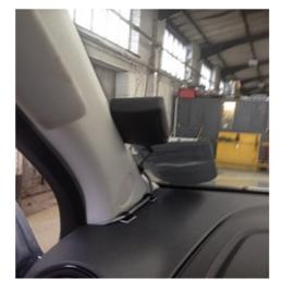
3. The GPS Module should be placed in a suitable area within the cab, preferably in an area next to the windscreen.
