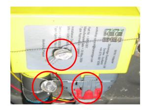
4. Seal the Connector and Sender to the Adaptor through the Red seal. Seal the Adaptor to the chassis of vehicle through 2 of the diagonal holes that have been drilled for securing the M1N1 Adaptor. Note: The M1N1 MUST be fixed to a non removable part of the vehicle.
