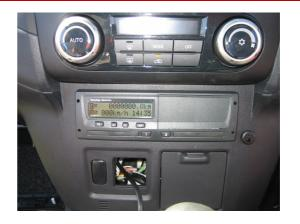
2. Install the tachograph into the slot. Ensure the tachograph can be removed from the enclosure with all cable connections attached.
