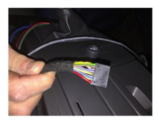
2. Suitable power, ignition and ground connections can be taken from the radio connector as shown above.
