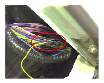
4. Solder and insulate this cable connection after first confirming and checking that speed is displayed on the SE5000 when vehicle is driven. Seal this connection and re-instate the conduit harness insulation. Secure all tachograph and M1N1 wiring and harnesses by routing along side existing cables.
