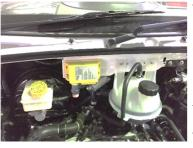
THE M1N1 ADAPTOR CAN BE MOUNTED AND SECURED TO THE METAL BULKHEAD PANEL UNDER THE BONNET, PICTURED LEFT. ROUTE CABLES THROUGH A SUITABLE BULKHEAD GROMMET TO VU LOCATION POINT. (EXCEPT FOR YELLOW WIRE FROM M1N1 ADAPTOR)
