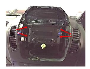
1. Remove the front cover panel to gain access to the four screws to remove the radio, as shown above.
