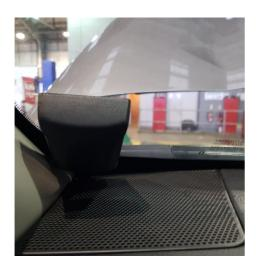
3. The GPS Module should be placed in a suitable position within the cab, preferably in an area next to the windscreen.
