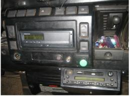
IMAGE LEFT SHOWS SE5000 TACHOGRAPH INSTALLED IN THE RADIO SLOT AND THE RADIO MOVED AND FITTED IN A MOUNTING TRAY. T-LIGHT (NOT INCLUDED) MUST BE FITTED IF VU LOCATION IS IN A DVSA DESIGNATED AMBER AREA. SEE SPECIAL NOTICE SN 2-2014
