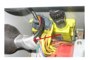
2. Secure the M1N1 with the 4 nuts and bolts provided in the kit. Feed all the harness wiring from the M1N1 through the shroud as shown. Route all cables and wires to the tachograph location point.
