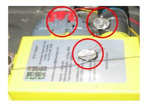
4. After performing the Initial Calibration, seal the Connector and Sender to the Adaptor through the Red seal and seal the Adaptor to the chassis of vehicle as the M1N1 must be fixed to a non removable part of the vehicle.
