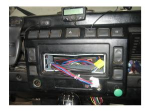
1. Locate the tachograph inside the radio slot on the centre console as shown. Ensure that a T-Light (not supplied in this kit) is fitted if the SE5000 is fitted in a DVSA designated Amber location. SEE DVSA SPECIAL NOTICE SN 2-2014
