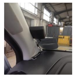
3. The GPS Module should be placed in a suitable position within the vehicle, preferably in an area next to the windscreen.
