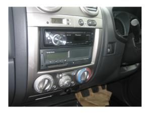
3. On some vehicles a new facia may be required. If the VU is not fitted as above and is in a DVSA Amber location you are required to fit a T-Light (not included in this kit). See Page 4 of this application sheet for fitting instructions.
