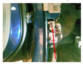
4. Locate the 2 block connectors behind the passenger kick panel as shown Connect D6 from the tacho to the BLACK wire YELLOW trace located on Pin 26 of top connector or it's sometimes on Pin 13 of bottom connector.
