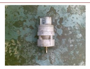
1. Completely remove the existing speed sensor including the drive key.
