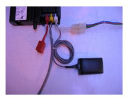
2. The cable harness is connected directly in line with the tachograph power cable when connecting to the tachograph as shown.
