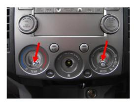
**4.** Remove original CD facia by removing the 3 knobs, then removing the 2 screws.
