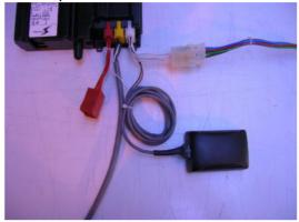
**22**. The cable harness is connected directly Inline with the tachograph power cable When connecting to the tachograph as shown.
