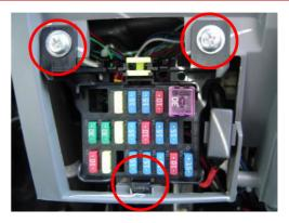
11. Remove the fuse box by unscrewing the 2 screws and unclipping the clasp at The bottom.
