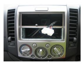
Install the tachograph cage before Clipping on the new facia and ensure the 2 screws are secure before replacing the knobs.
