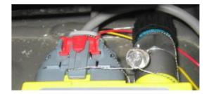
**20**. Seal the sender and connector Through the Red Seal provided to the Adaptor.
