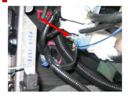
**13**. The Ground connections for A5 and A6 of the tachograph can be picked up from the common ground bolt near the accelerator.
