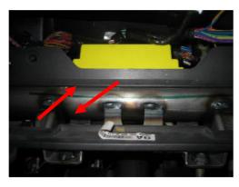
3. The Adaptor must be sealed to a non Removable part of the vehicle. Use the Cross frame bar to loop the sealing wire around.
