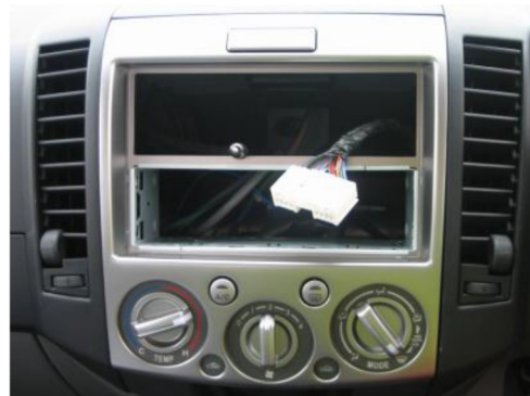
15. Install the tachograph cage before Clipping on the new facia and ensure the 2 screws are secure before replacing the knobs.
