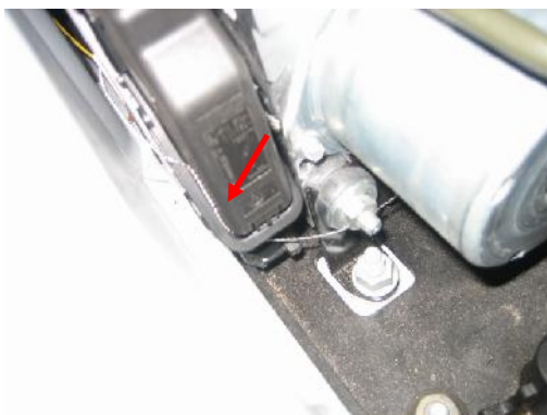
11. Connect the ABS connector and seal using sealing wire like the example above, ensuring that the connector cannot be removed.
