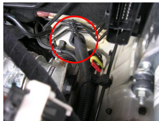
10. Feed the wires from the M1N1 through the grommet into the cab.
